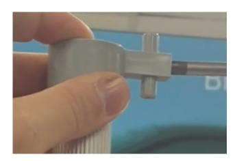
**Step 3**Fix the other 2 clips to the top of each pole with the screw located at the side. This will secure the clip at this height.
